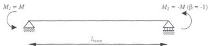
Fig. 9 - Beam subjected to a moment distribution described with \beta = -1
