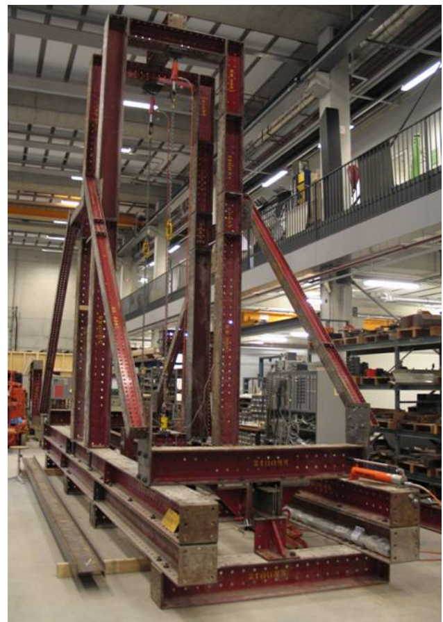
Figure 2. Test set-up for test 1 without concrete slab.
